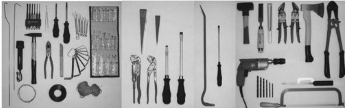
Pic.3. The tools used to test doors to burglary resistance class 4 (WK4) by EN-1627.
