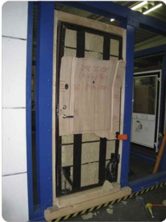
Pic.1. External opening door test
