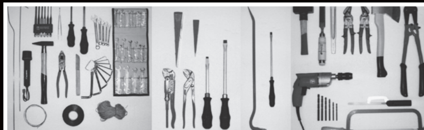
Tools used for testing 4th security class doors.
