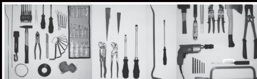
Tools used for testing 4th security class doors.
